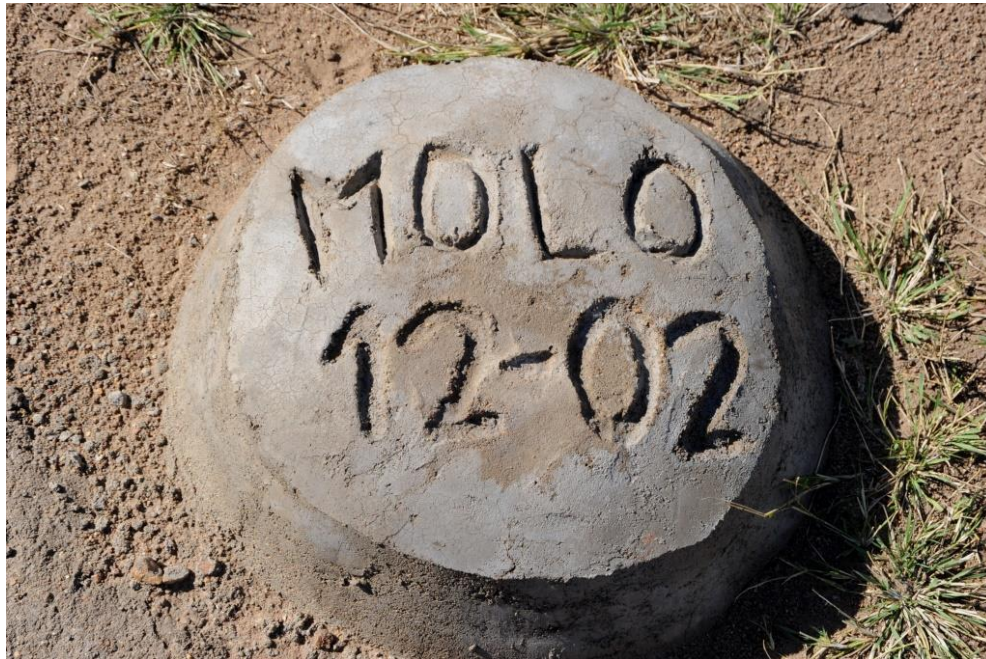
Figure 21: Concrete Marker Showing the Collar Position of Borehole Molo 12-02
