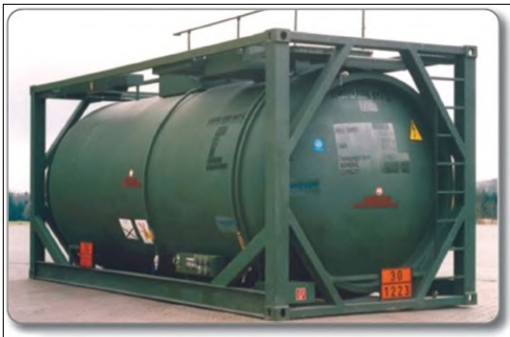
Figure 79: Typical Layout of Containerized Fuel Storage Tank
